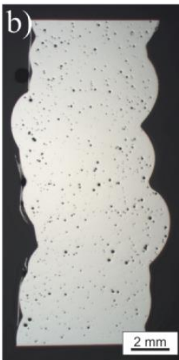
Figure 5: Unetched cross section of MA-6063 WAAM sample [1].
