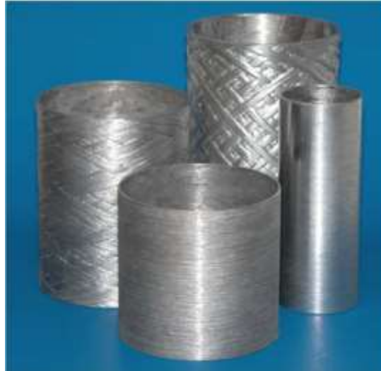
Figure 4: Open ended wet filament wound AMC cylinders as produced by MetPreg 47
