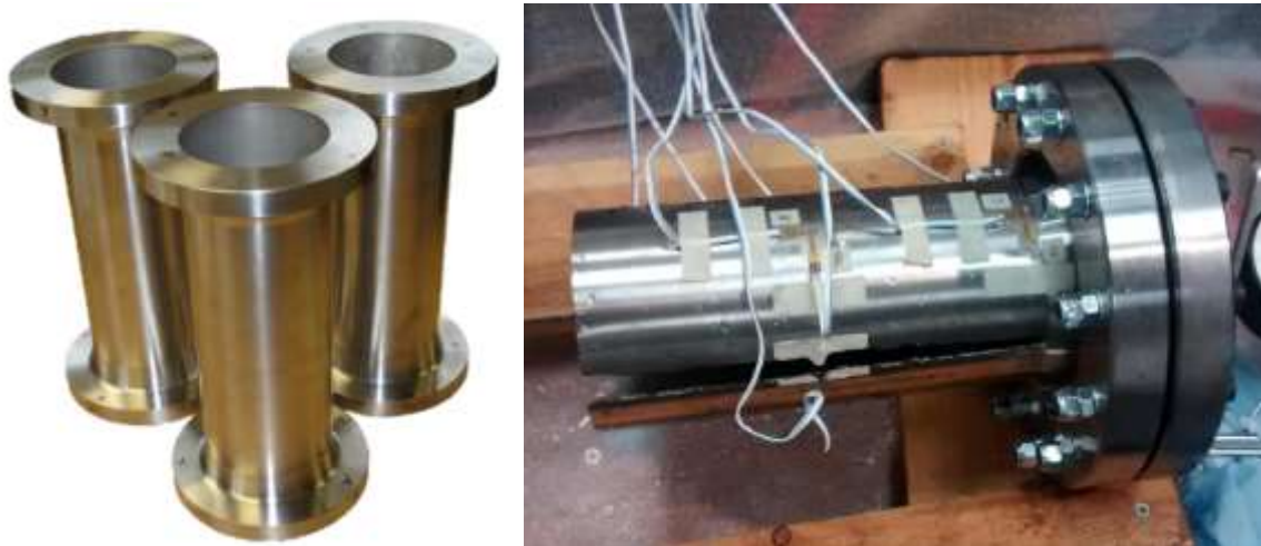
Figure 6: TISICS MMC pressure tube, left) pretesting pressure tubes, right) pressure tube after failure 49
